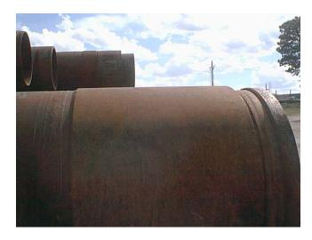
The action of the larger diameter of the drill collars as catch points is illustrated by using the thumb and first finger on one hand to grasp before the knuckles of the fingers on the other hand. The larger size of the knuckles form catch points. The large collars were not necessary. Threaded collars with the same dimension as the drill casing are available and had adequate strength for the drilling activities.
