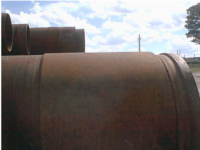
Figure 2. The Large Threaded Connectors on the LANL Retractable Drill Casing Increased the Potential for the Casing to Become Seized in Boreholes.
