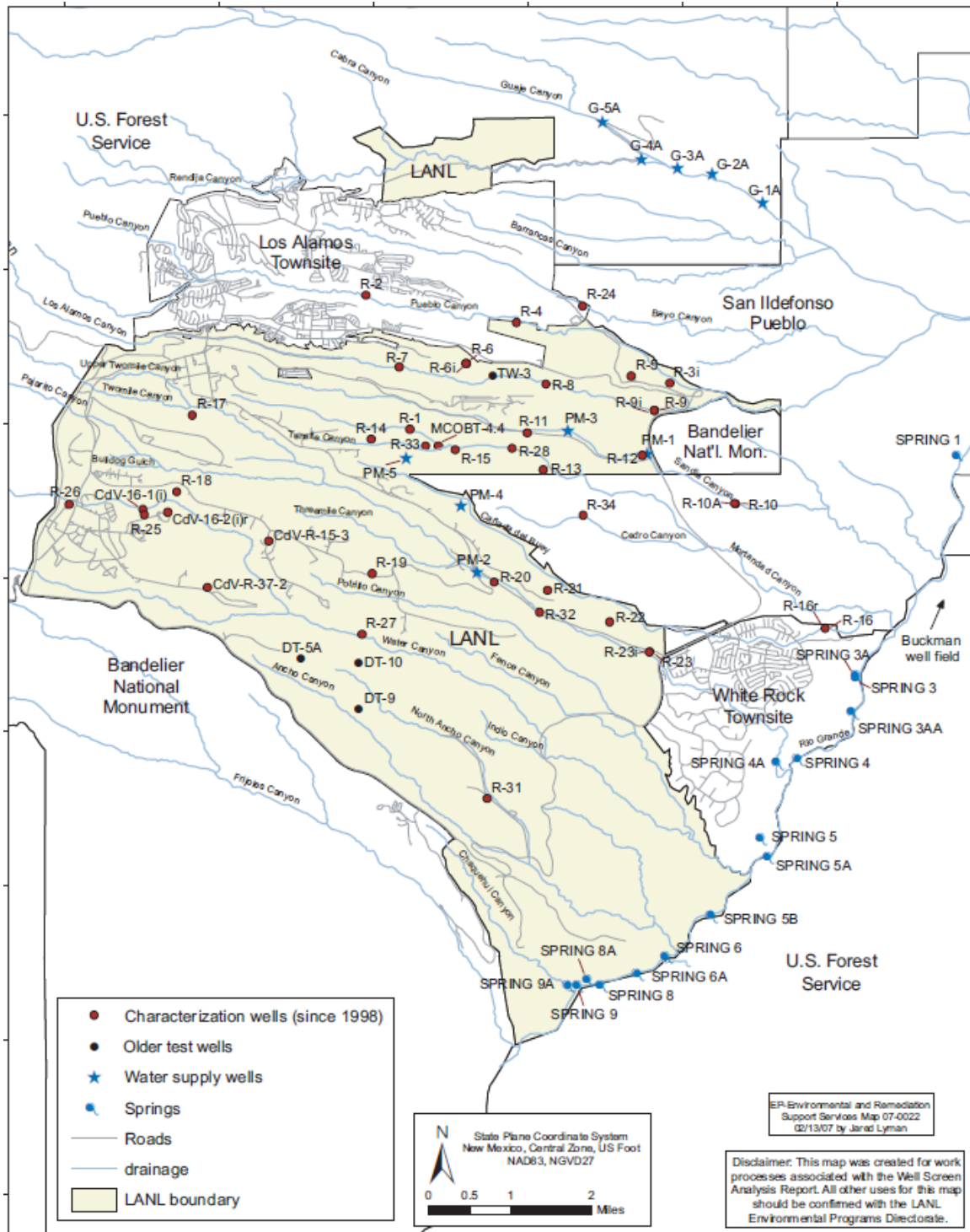
Figure 4. The network of monitoring wells and drinking water supply wells at the Los Alamos National Laboratory.
