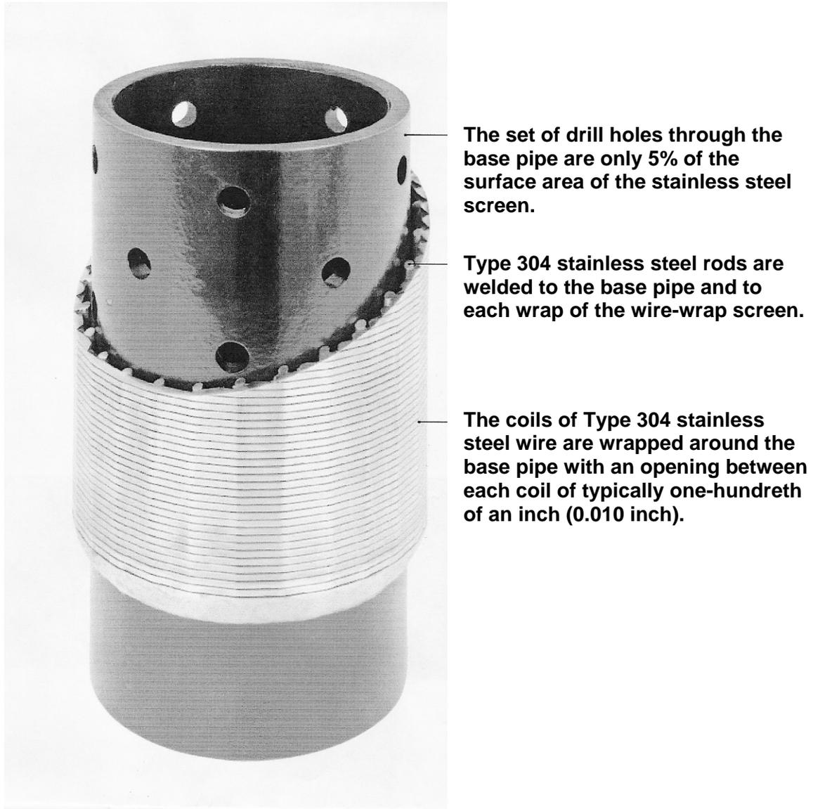
The constrictive design of the pipe-based screens prevents efforts at well rehabilitation from even cleaning residual drilling additives and clays from the wire wraps of the well screens. Deep cleaning of the new mineralogy produced by the drilling additives from the filter pack that surrounds the well screen and from the zone surrounding the borehole is not feasible.
